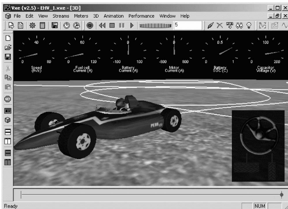
Fig. 5. Three-dimensional visualization of the performance of an electric vehicle, including dashboard instruments, and steering wheel for user interaction.
